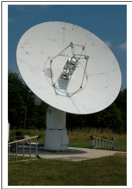
Figure 1: VLBI2010 broadband receiver mounted on 5-m MV-3 antenna at GGAO. MV-3 will be replaced by a 12-m VLBI2010 antenna.
